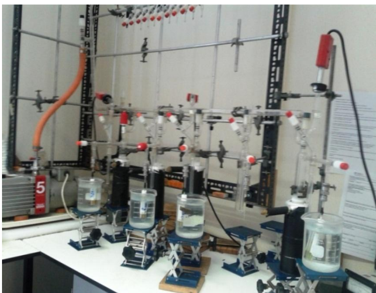
Figure 4.5 Extraction and distillation of water by vacuum manifold with five units
