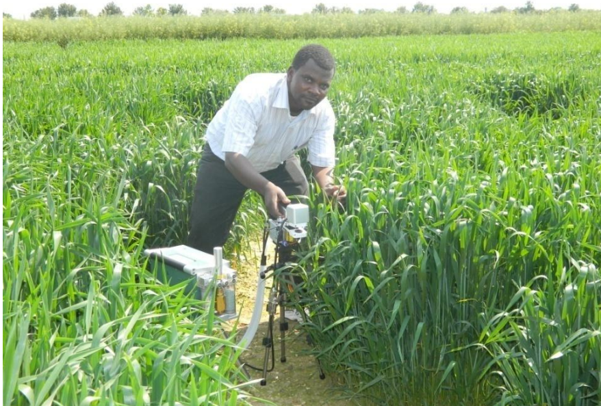
Figure 2.2 Gas exchange measurement in the field with LI-COR
