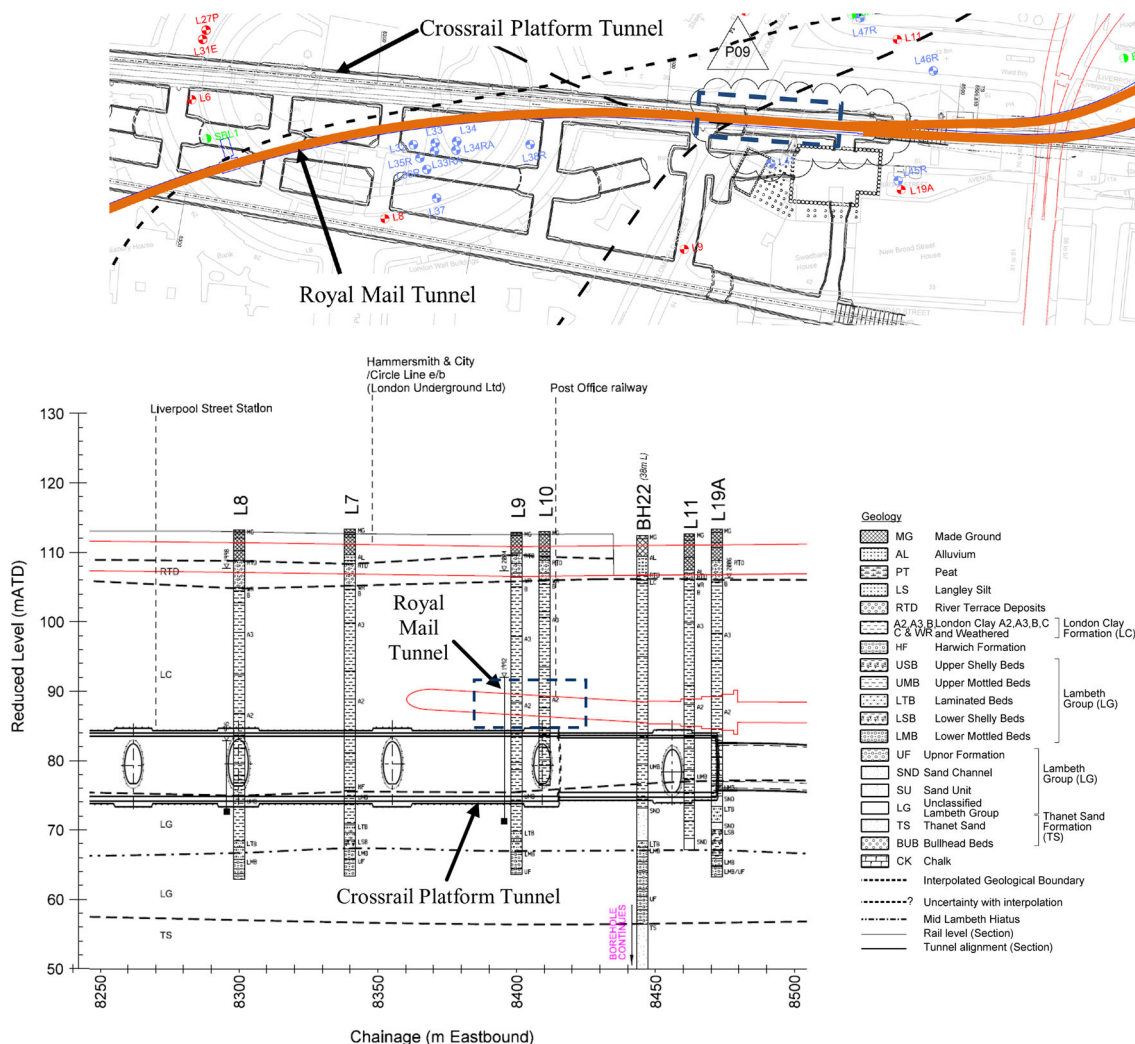
Fig. 1 (Top) alignment of Royal Mail tunnel and Crossrail platform tunnel at London Liverpool Street Station. (Bottom) longitudinal section view of Royal Mail and Crossrail platform tunnel with soil profile
