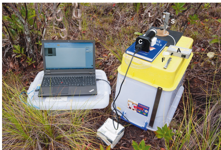
Figure 12 Seymour device in field testing. Labels: C – camera; L – lens; S – Seymour extensional rheometer; F – feeler gauges; A – solenoid switch.
