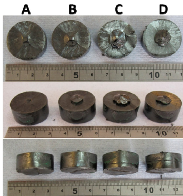
Figure 3. Top and side views of TSMG processed YBCO sample A (with no buffer pellet) and samples B, C, and D (fabricated with different buffer pellets).
