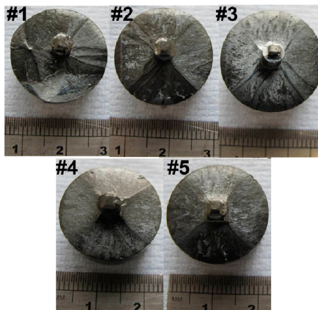
Figure 11. Top view of the TSMG processed YBCO samples #1, #2, #3, #4, and #5 with buffer pellets of different aspect ratios (3.0 to 1.1).
