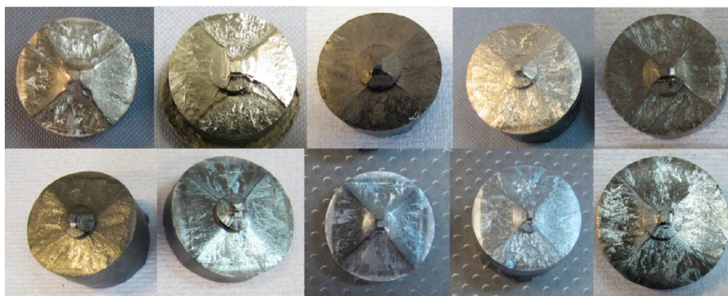
Figure 14. Photographs of a batch of YBCO samples fabricated using capped buffer pellets. Single-grain growth of the Y-123 phase is indicated by the presence of the four facet lines in each sample.
