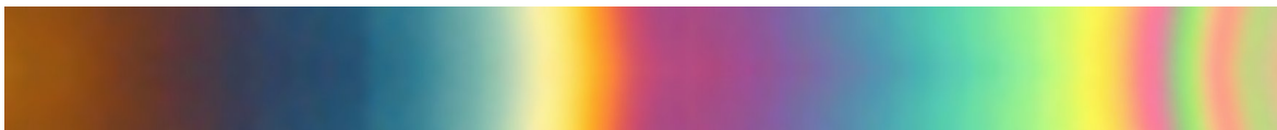
Figure 3.5: Interference colours from a thickness gradient in a PS film on a silicon wafer, with refractive indices of 1.6 and 4.1, respectively. (Reproduced from [127]). Starting from brown (20 nm) on the left, through light purple (400 nm), pink (520 nm) and eventually to alternating light green and pink ( \sim 1.5 \mu\text{m} ), the color eventually changes to a transparent grey for very thick films.
