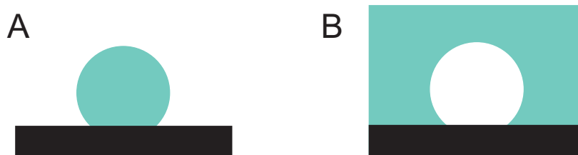
Figure 7.1: (A) Wetting of a solid surface by a liquid drop in a vapour environment. (B) Wetting of a solid surface with a vapour bubble in a liquid environment.
