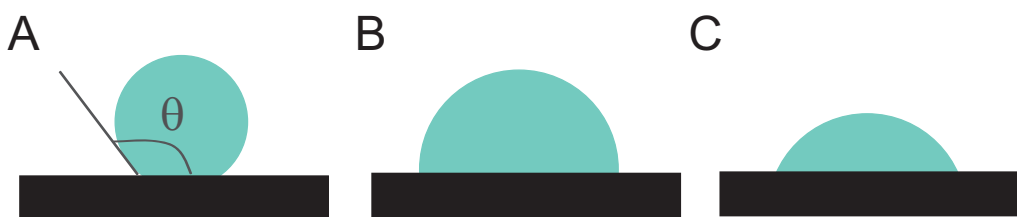
Figure 7.2: Contact angle \theta_Y of water on (A) a hydrophobic surface ( \theta_Y > 90^\circ ) (B) a neutral surface ( \theta_Y = 90^\circ ) (C) a hydrophilic surface ( \theta_Y < 90^\circ )
