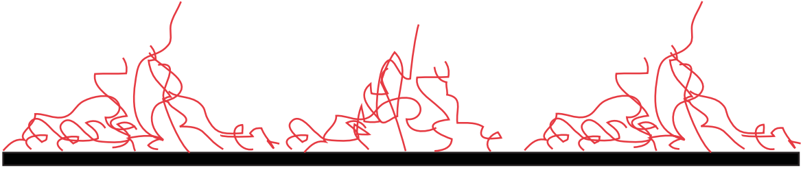
Figure 5.3: The expected deformation of a molten polymer brush under an applied electric field. The surface grafting limits the lateral mass transport in the film during instability formation.
