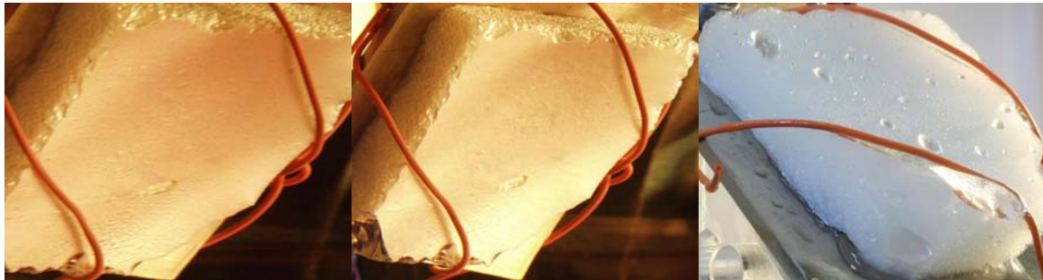
(a) Plastron (10 days in H 2 O) (b) Plastron (21 days in H 2 O) (c) Wet surface after removal
