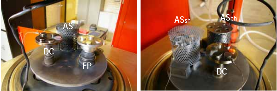
Figure 3.2.1-3: DC, AS sh , AS bh , and FP arrangements inside a conventional DC plasma furnace used to study the mechanisms of active screen plasma treatments. DC: direct current; AS: active screen; FP: floating potential; AS sh : AS mesh with small holes (Ø = 8 mm), AS bh : AS mesh with large holes (Ø = 25.4 mm)
