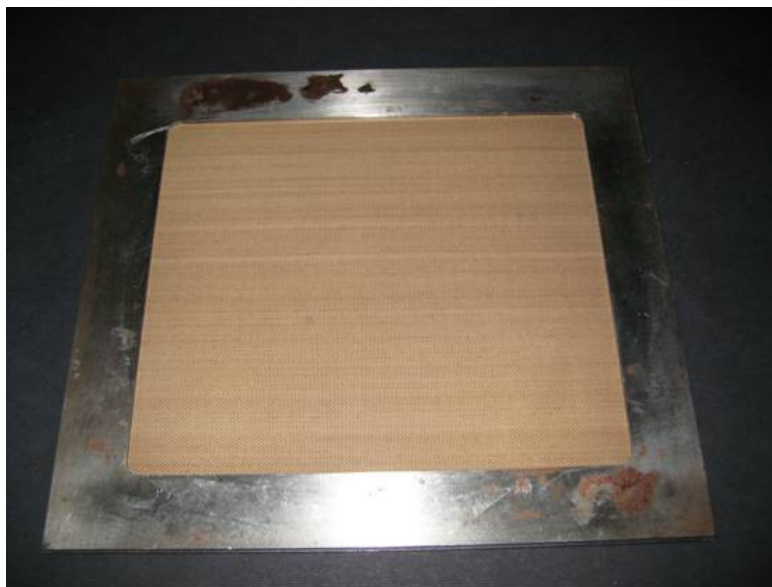
Figure 3.11: Mould lined with PTFE sheets.
