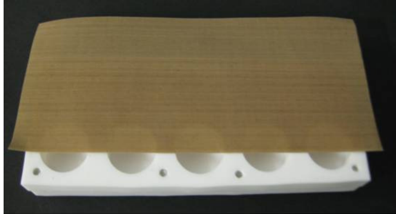
Figure 3.6: Cylindrical mould with PTFE sheet.
