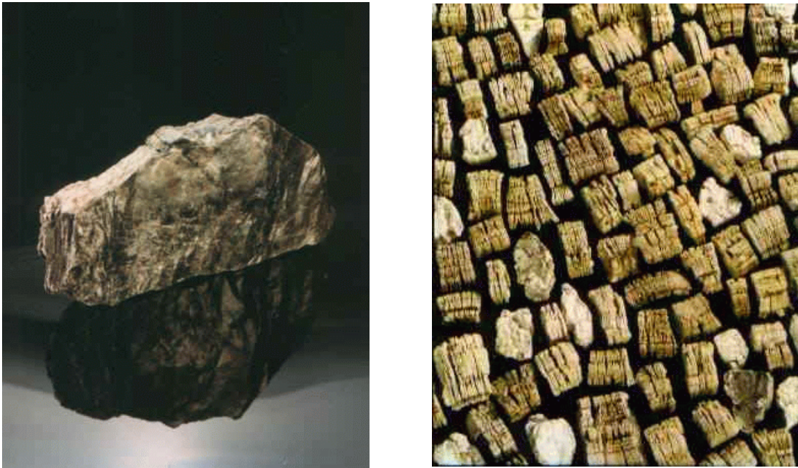
Figure 7.1 : Shown above left is an unexpanded vermiculite “book” with some exfoliated “books” shown on the right [Mandoval Ltd, 1999].
