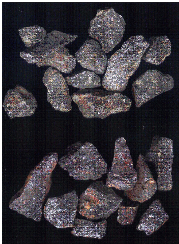
Figure 6.1 : A digitised scanned image of particles from S1 (top) and S2 (bottom). S2 exhibits a darker, more metallic grey colour as well as a greater degree of oxidation than S1.
