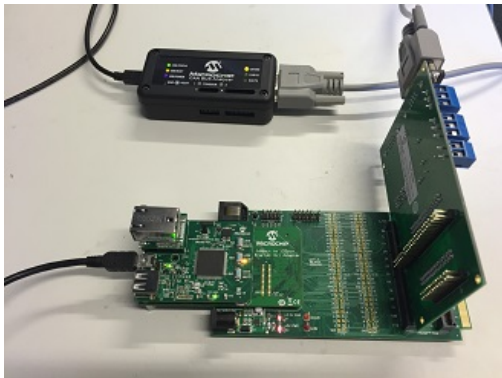
Fig. 4. Lab setup for CCU’s CAN bus communication
