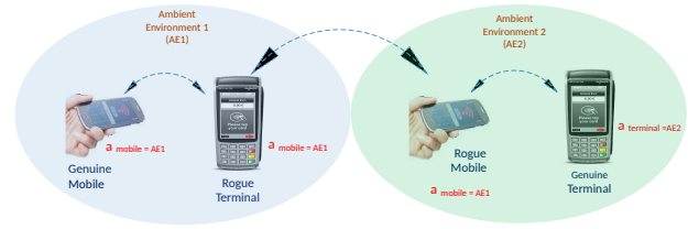
Fig. 4. Ambient Sensing as a Token Relay Attack Prevention Countermeasure
