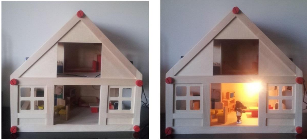
Picture 6-1. Miniature Smart home before and after the UA has detected presence.
