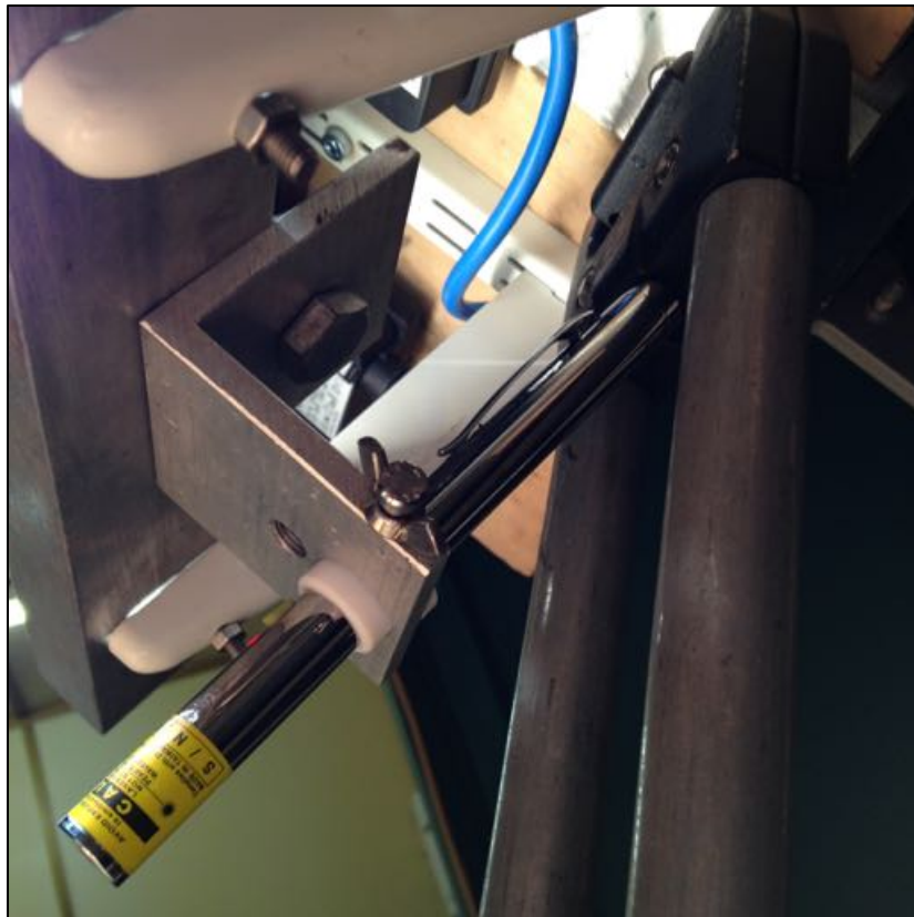
Figure 3.15. Laser pointer attached to the base of the lamp mounting board
