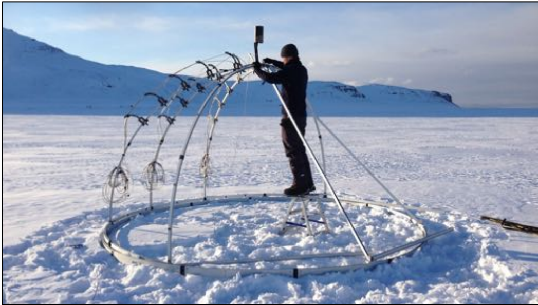
Figure 2.3. Construction of the goniometer's frame at the field site
