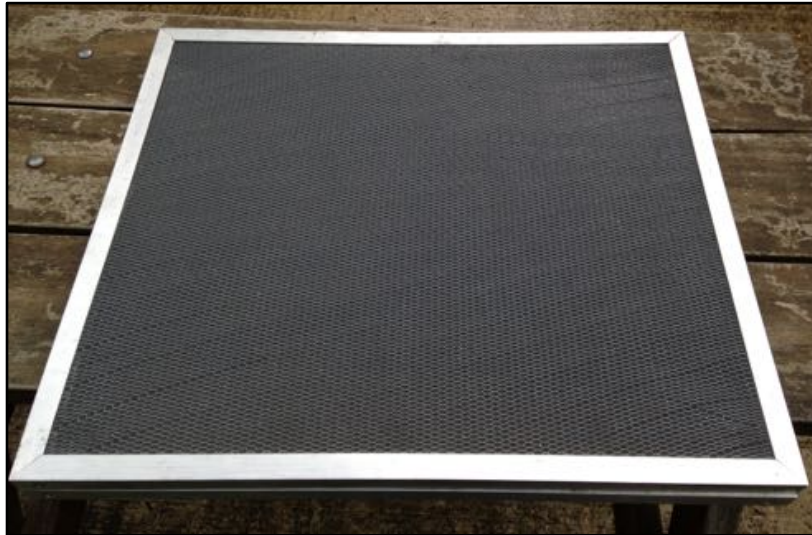
Figure 3.17. Baffle made of aluminium mesh in a honeycomb structure
