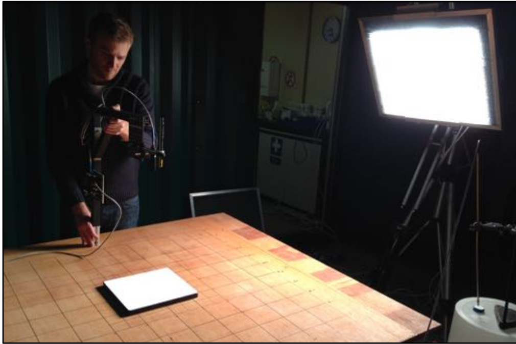
Figure 3.20. Experiment to characterize the footprint of the lamp array
