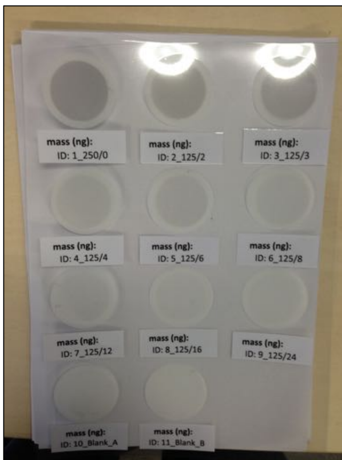
Figure 2.13. Photograph of field reference filters used to estimate the maximum black carbon mass ratios in snow at the field sites
