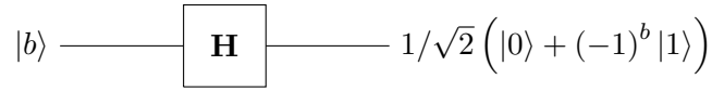
Figure 3.1: Schematic representation of H gate operating on a qubit in state |b\rangle
