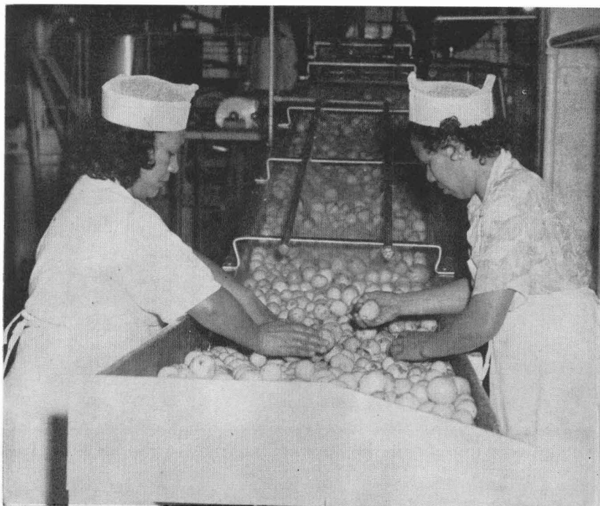
FIGURE 2. Inspecting and washing of whole guavas before processing. (Courtesy Hawaiian Juice Industries, Ltd.)
