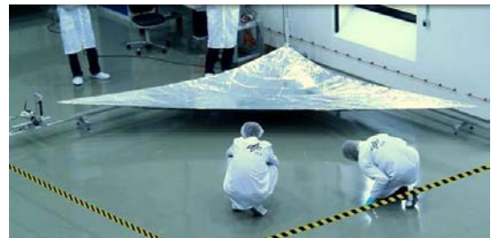
Figure 20: Deployment test of one sail segment alone without booms and BSDU.
