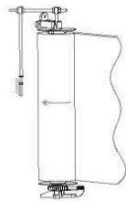
(b) Uncoiling sail segment from spool.
