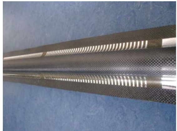
Figure 12: Reflective marker on the boom. An optical sensor determines the deployment process by scanning the markers.
