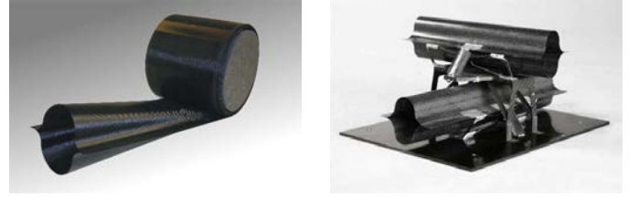
(a) Photograph of a partially stowed boom with larger cross section compared to Gossamer-1. (b) Boom Spacecraft Interface for two crossed booms with vertical displacement.
