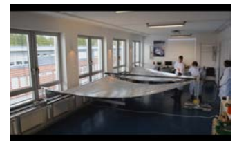
(b) Sail completely deployed, BSDU separation - Phase 5.
