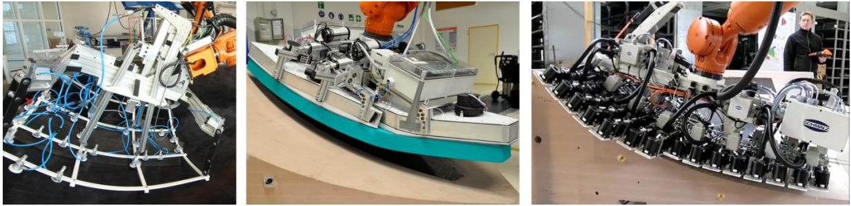
Figure 7: Hardware demonstrators of three preforming grippers (from left: Grid Gripper, Foam Gripper, and Modular Surface Gripper)
