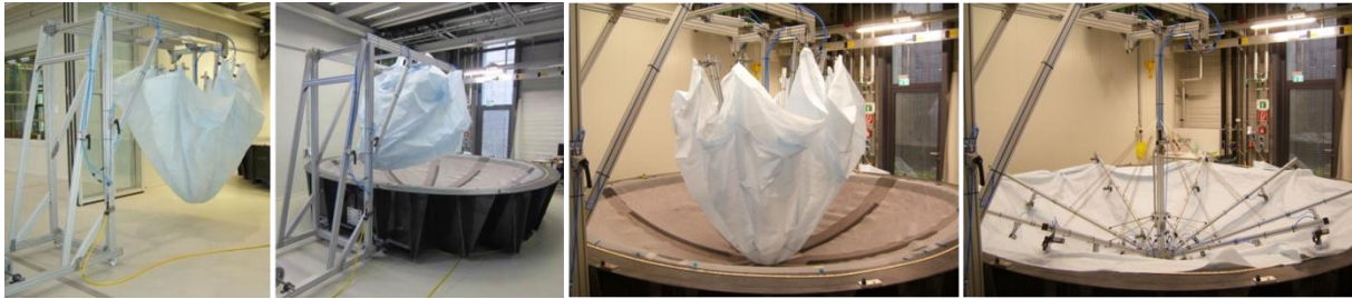
Figure 16: Semi-automated lay-up process for infusion membrane
