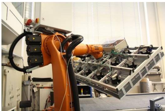
Figure 5: Flexible robot-based end-effector for handling and draping of textile cut-pieces, Fraunhofer IWB, ref. [3]
