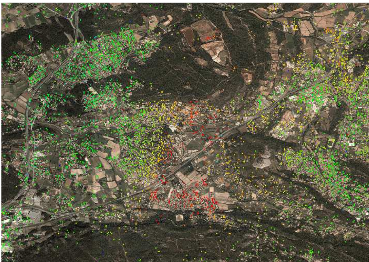
Figure 9: Data plotted on top of an aerial photo (obtained via maps.google.com). No correction is made to shift the background image such that it aligns best with the geo-referenced displacement rates. This image illustrates the point density in the subsidence area and possibilities of GIS/geoTIFF interface.
