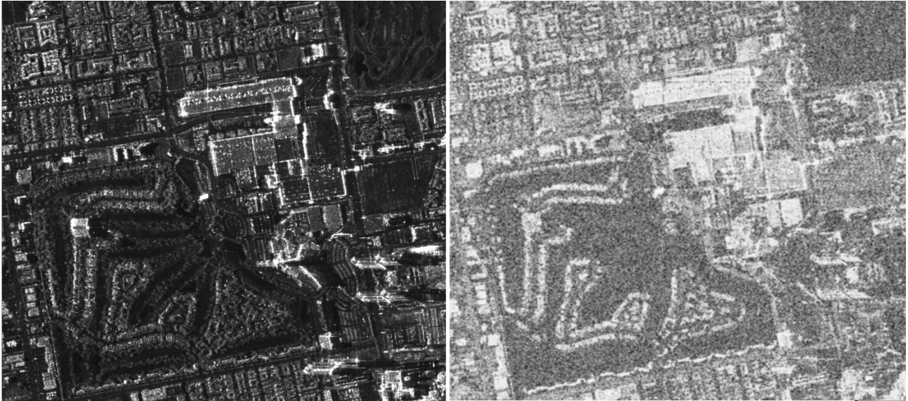
Fig. 12: Crop from the spotlight test site Las Vegas covering the Convention Center building; left: mean intensity radiometric enhanced by 8 temporal looks; right: the coherence estimate indicates a high phase stability on the man made features (e.g. the building's roof)
