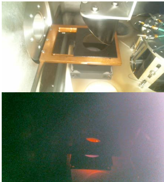
Figure 3. Current test configuration in the chamber – TOP: Sample at 450°C illuminated by a LED panel in the chamber, BOTTOM: Same scene without additional light.
