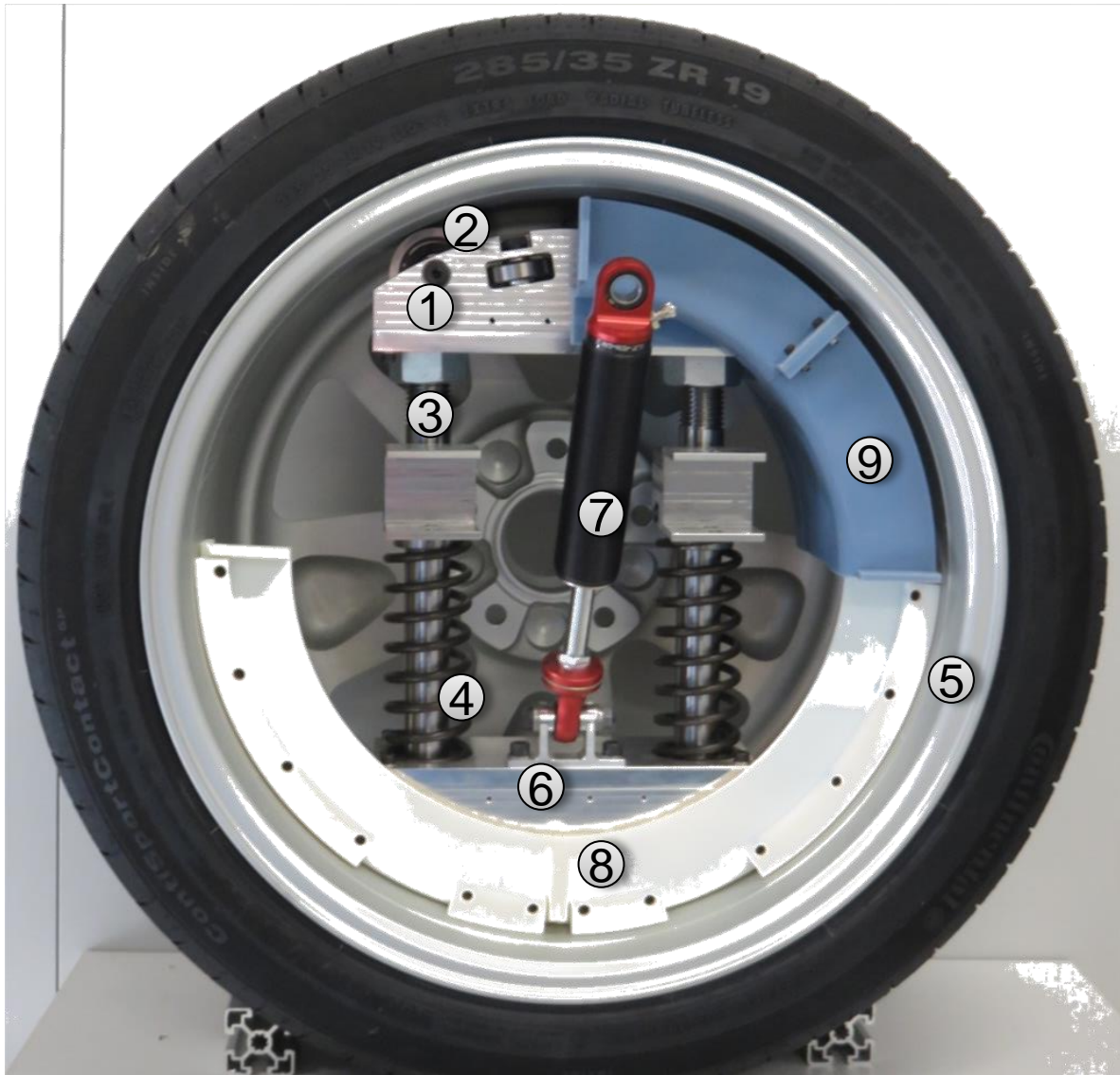
Figure 6: First prototype of the innovative in-wheel suspension LEICHT : wheel guidance, springing, damping, bearings and sealing is shown
