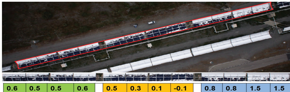
FIGURE 6: Aerial image of three SCAs, with corresponding ortho image and estimated relative module misalignment in ^{\circ} . The right part of the central SCA is oriented almost exactly towards the camera, while the left and the right show pronounced deviations. Possible reasons for the observed deviations are offsets of the tracking system, friction and misalignment between SCEs.
