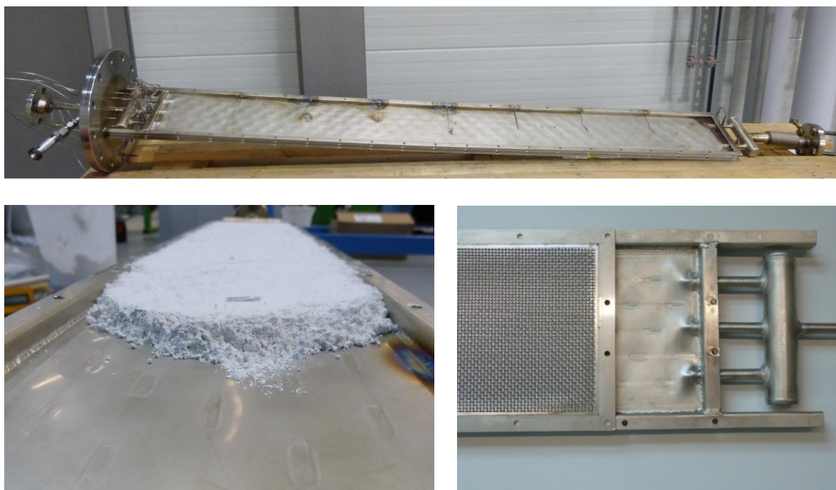
126 Fig. 2 Top: heat exchanger plate used as reactor; bottom left: storage material filled into the frame; 127 bottom right: filter plate to encase the reaction bed
