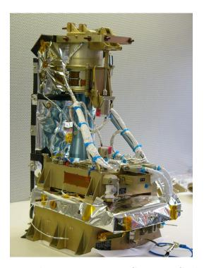
Figure 2.6.: The Dawn Framing Camera. Credit: MPS.
