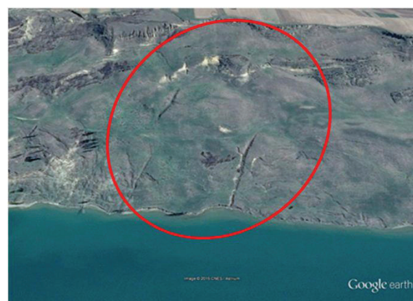
Figure 8. Closer look at the active landslide area identified in Figure 2, showing clear evidence of ground instability in Google Earth imagery
