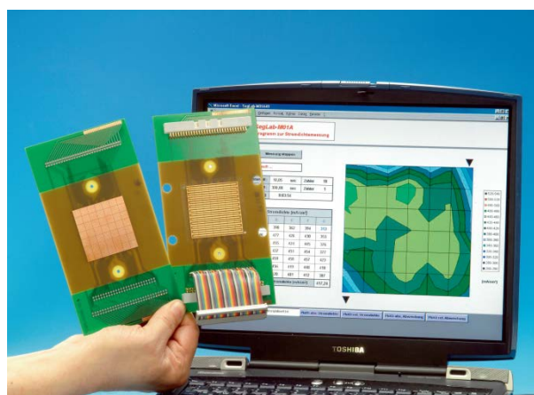
Figure 1. Segmented printed circuit boards for in-situ online-diagnostics in PEM fuel cells
