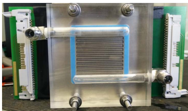
Figure 2. Successful integration of segmented PCB in PEMWE test cell with optical access
