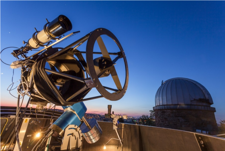
Figure. 6.1.1: The DLR ground station in Stuttgart, Germany will perform link budget measurements to satellites using a pulsed Nd:YAG laser (1064nm, 3ns, 3kHz) as source and an InGaAs based SPAD as detector.
