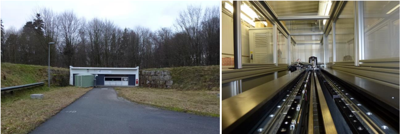
Figure 2. Left: View of the receiver station with open gate. Cage of the agile target platform is open in transmitter direction. Right: Sliding carriage system of agile target platform within the cage. A traveling distance of 1.7 m can be used.
