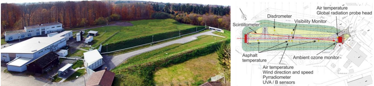
Figure 1. Left: Aerial photography of DLR laser test site in Lampoldshausen with transmitter station, test range and receiver station. Right: Different types of environment measurement systems and their position to monitor selected parameters 24/7.
