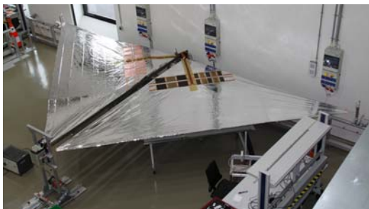
Fig. 18. EQM fully deployed during deployment test preparation
