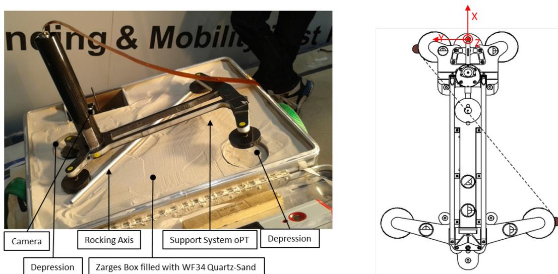
Figure 8 Left: Overview of the test setup of the Rocking Test. Right: Schematic topview with rocking axis and coordinate system
