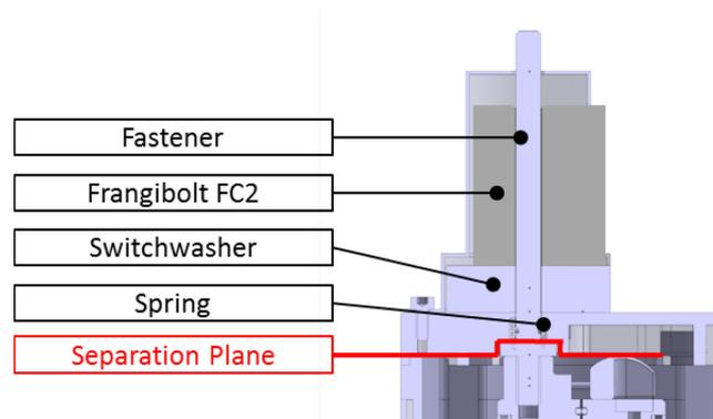
Figure 4 Overview of the Mole to Support System separation mechanism
