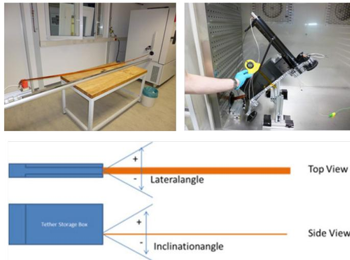
Figure 5 Overview of the Test setup for the Engineering Tether Pull-out test and the pull-out angles
