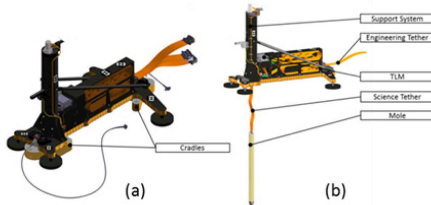
Figure 1: Overview of the HP<sup>3</sup> configuration. Left: Undeployed configuration on the lander deck. Right: Partially deployed configuration
