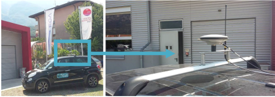
Figure 15.6: Antennas of the RTK rover station mounted on the CRF car rooftop
