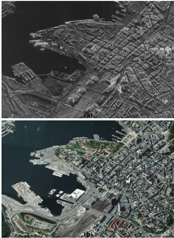
Figure 5: SAR image of the Oslo city center in slant-range geometry (a) and co-registered optical image (b).
