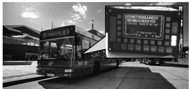
Figure 7. Bus driver display shows requested assistance
