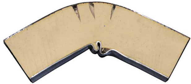
Figure 12. Sectional view of the foam-filled steel beam S40S in three-point bending tests [30].
