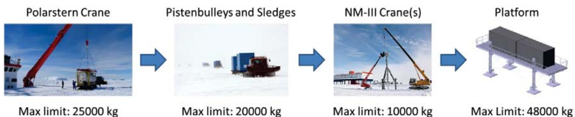
Figure 15. Polarstern crane, Pistenbully/sledge, Neumayer III crane and platform mass restrictions (Credit for small photos: AWI).
