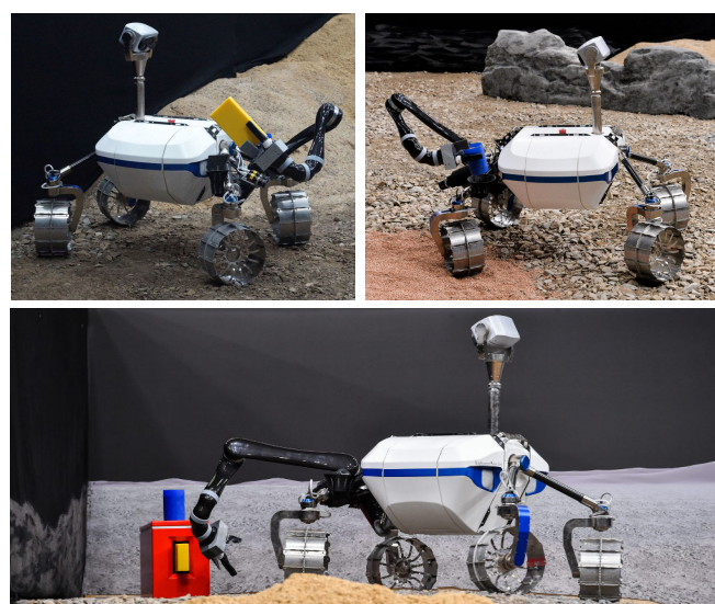
Fig. 1. The Light Weight Rover Unit (LRU) picks up the battery (yellow, top left) and the sample (blue container, top right) and assembles them at the base station (red, bottom) during the SpaceBotCamp challenge.
