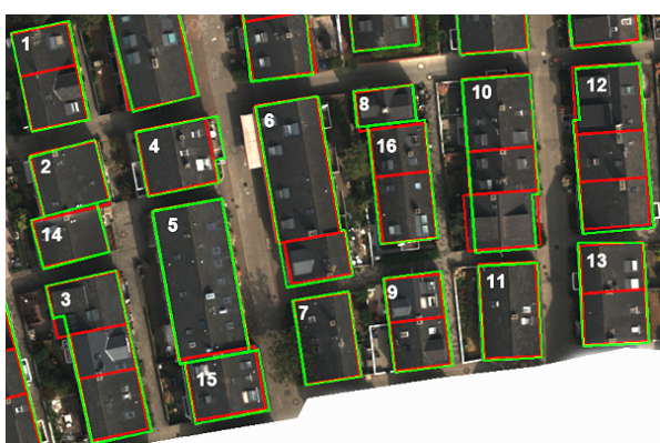
Figure 4. Accuracy of reconstructed building footprints (green) compared to the ALK (red) neglecting inside walls
