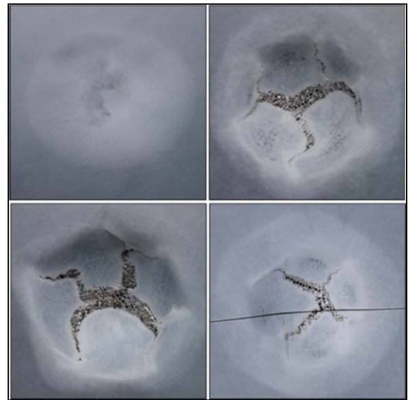
Fig. 14: Impacted area of Test 1 (top, left), 2 (top, right), 3 (bottom, left) and E2 (bottom, right)
