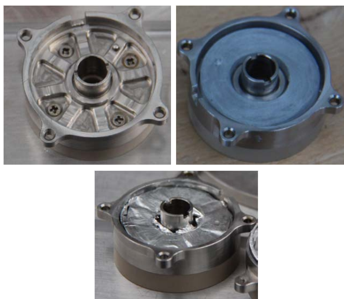
Fig. 3-6: Upper Collection Pan Assembly with insulator
