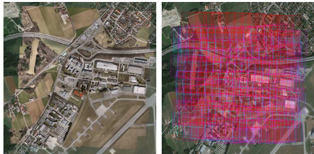
(b) satellite image augmented by orthorectified and tessellated nadir images (c) footprints of complete image sequence: nadir (red), forward (magenta), and backward (cyan) looking camera
