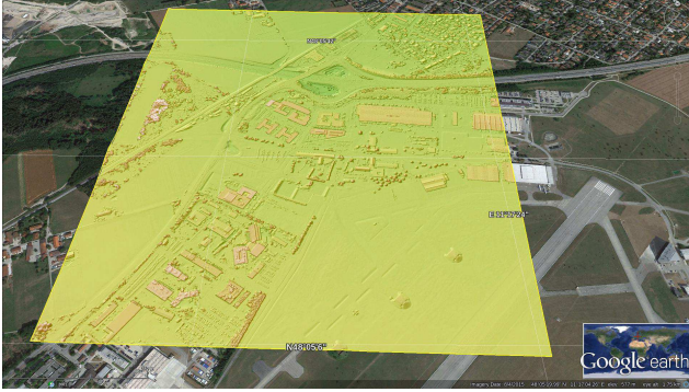
Figure 9: A digital surface model (DSM) generated from the DLR-3K aerial image sequence.
