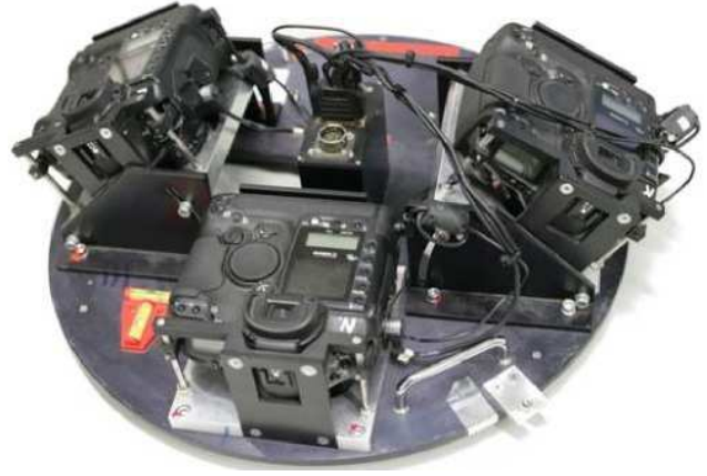
(a) the DLR 3K sensor setup uses 3 DSLR cameras with different viewing angles
