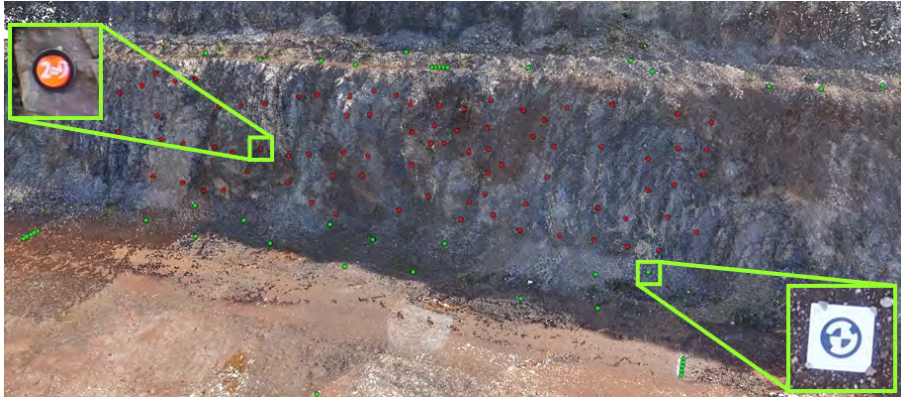
Figure 13: The reference point network allows an extensive accuracy evaluation. Markers (right) indicating GCP positions are shown in green, circular targets (left) for quantitative evaluation are in red.
