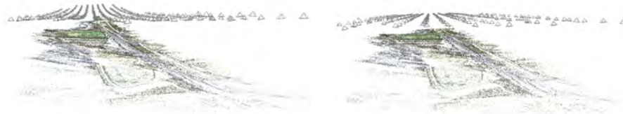
Figure 7: Results of the photogrammetric reconstruction without (left) and with additional GPS positions and optimization of camera intrinsics in the bundle adjustment (right). The direct comparison shows the reduction of the initially clearly visible distortion of image block and object points.
