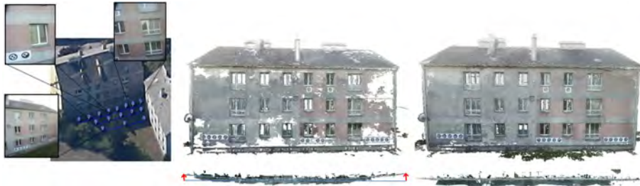
Figure 9: Left: Graz500 multi-scale facade dataset. Middle: The reconstruction of a facade computed with a well-known state-of-the-art method [33] shows, though visually correct in appearance, holes and geometric inconsistencies (significant bends along the fringes). Right: In comparison, using our multi-scale approach and online feedback support results in a straight wall and complete scene reconstruction.
