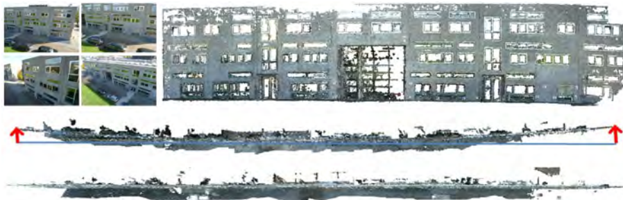
Figure 4: In the facade reconstruction using OpenCV calibration significant bending is prevalent (middle). In contrast, accurate camera parameters delivered by our method [14] results in a straight facade reconstruction (bottom).
