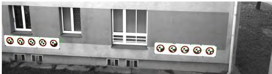
Figure 11: Automatically detected ground control points with plotted marker centers and corresponding marker IDs.
