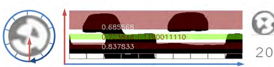
Figure 3: Histogram for an unrolled circular marker and rotation invariant binning of the code stripe. The numbers from top to bottom indicate the probabilities for center, binary code and outer circle. The marker with ID 20 has been successfully decoded.
