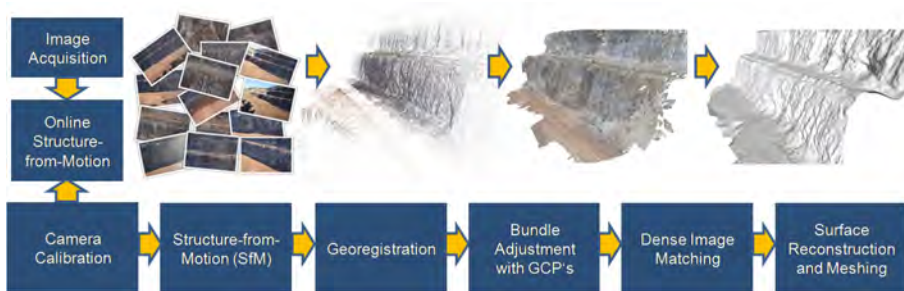
Figure 1: Automated processing workflow for geo-accurate reconstructions. Top row: Image set, sparse reconstruction, dense point cloud and triangle-based surface mesh of a quarry wall in open pit mining.
