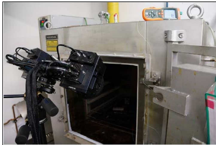
Figure 10. Stereo camera system placed in front of a furnace with a temperature-resistant and nonreflecting window.
