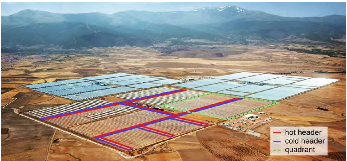
Figure 2.14: Aerial view from northeast of Andasol I-III PTC power plants with superimposed field and header structure (three loops are indicated) [20]
