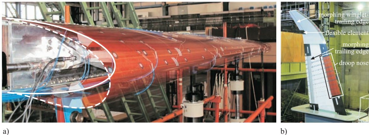
Figure 2. Full-scale testing of the DLR morphing leading-edge: a) 4 m span ground test 2015. The clean (white line) and drooped (dashed white line) configurations are shown. b) Full-scale test of an outboard section of a morphing wing at the t101 wind tunnel of TsAGI with the 3 m span morphing leading edge (box) and other adaptive, integrated systems.
