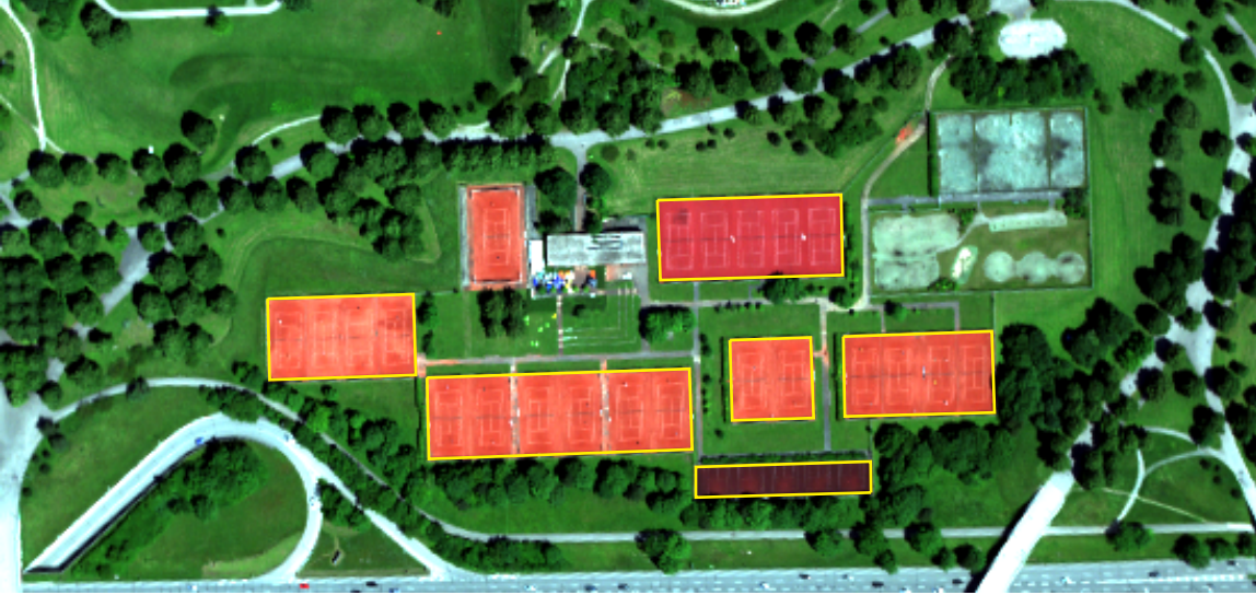
Figure 6.2: The tennis court test dataset with superimposed reference polygons. The RGB composite of the HySpex HSI is shown. The outer boundaries of the six clay tennis courts were manually digitised and are superimposed over the image (yellow). The most northern tennis court is excluded from the evaluation, because the clay material is spread around the tennis court. Consequently, the material boundary could not be reliably digitised.
