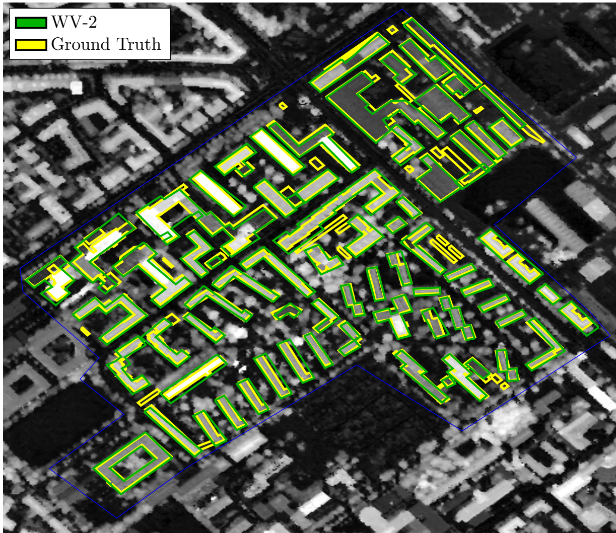
Figure 6.32: Adjusted BP extracted from WV-2 DSM (green) with GSD = 2.0 m ( large area ). Due to the roof overhangs, which are not included in the ground truth BP (yellow), the adjusted BP are in general larger than the ground truth BP.
