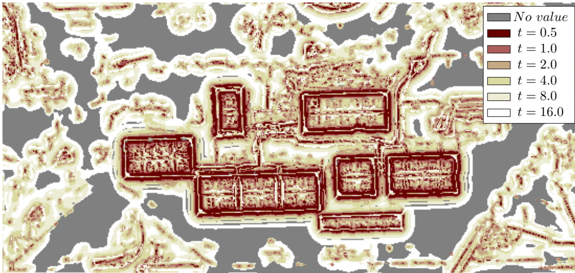
Figure 6.3: Selected scale t_{max} \in \{0.5, 1.0, 2.0, 4.0, 8.0, 16.0\} on the basis of maximal edge probability for tennis court dataset. The scales span from the finest scale ( t = 0.5 , dark red), over middle rang scales ( t = 4.0 , yellow) to the coarsest scale ( t = 16.0 , white). The edge probabilities are computed from the derivatives. If the the derivatives are considered unreliable (Equation (18)), the edge probability is set to zero. Thus, these pixels have no corresponding selected scale and are labelled as “no value” (grey).
