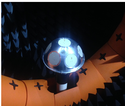
Fig. 3. The conformal antenna array in a measurement chamber at the DLR.
