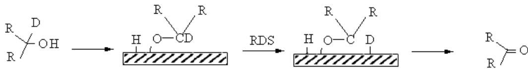
Figure 2.1) Proposed mechanism for the oxidation of alcohol (Van den Tillaart, Kuster et al. 1994).
