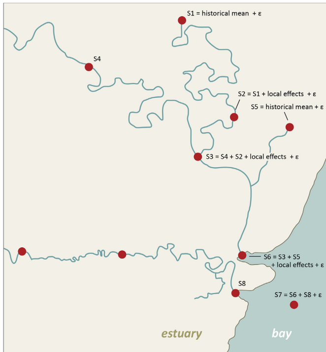
Fig. 3. Biophysical model. Each site represents an EHMP monitoring station. Site S1 is an uppermost estuarine station in a catchment. Site S2 is affected by S1, but also by local management actions. Further downstream at the river mouth, site S6 is affected by several sites (S3 and S5) as well as local effects. In the bay, sites, such as S7, are influenced in some way by sites at the mouths of the estuaries. At each EHMP station, the effects from local management actions and changes from upstream stations are propagated with consequential cumulative effects across the network (Dutra et al., 2010). A random component \epsilon is introduced at all sites to represent the variability seen in the historical data. Locations and densities of EHMP stations in this example are fictitious.
