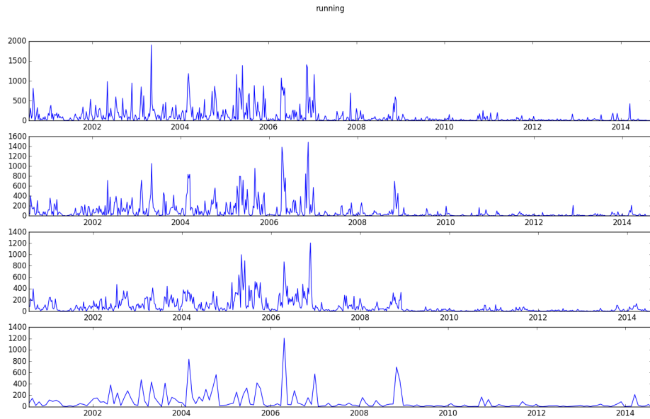
Figure 7.1: Graph of intensity of periodicity for running. Panel A is intensity graph computed with window size 14 overlapping size 7. Panel B is intensity graph computed with window size 28 overlapping size 21. Panel C is intensity graph computed with window size 70 overlapping size 63. Panel D is intensity graph computed with window size 28 overlapping size 0. X axis is time and Y axis is periodicity intensity.
