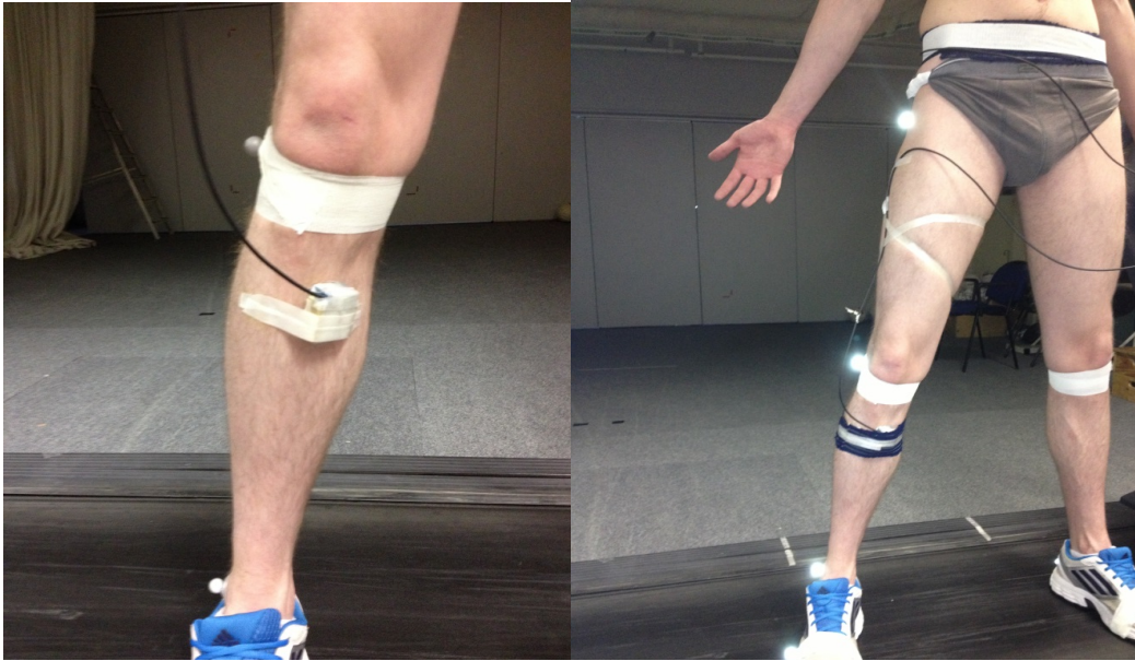
Figure 4.2 4: Anatomical position of tibial accelerometer (right), preloaded accelerometer attached with elastic Velcro strapping and reinforced with zinc oxide tape (right)
