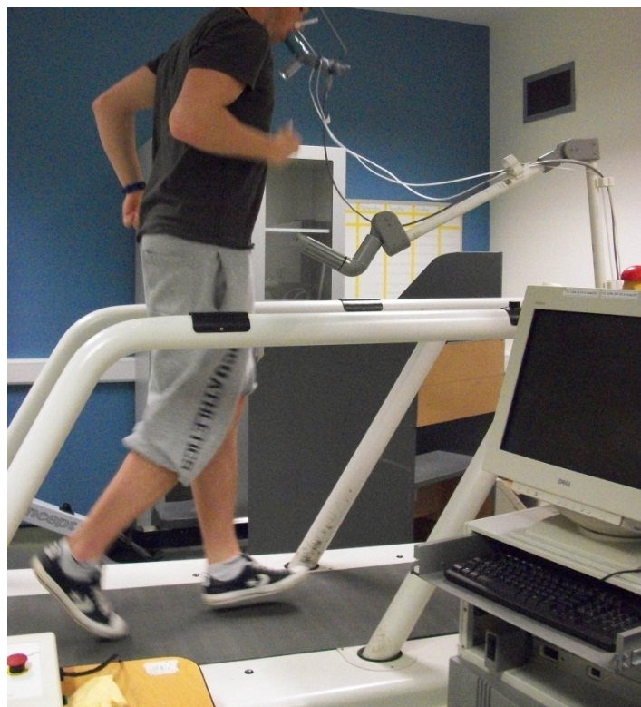
Figure 3.2. 5:Gas flow sensor and monitor
